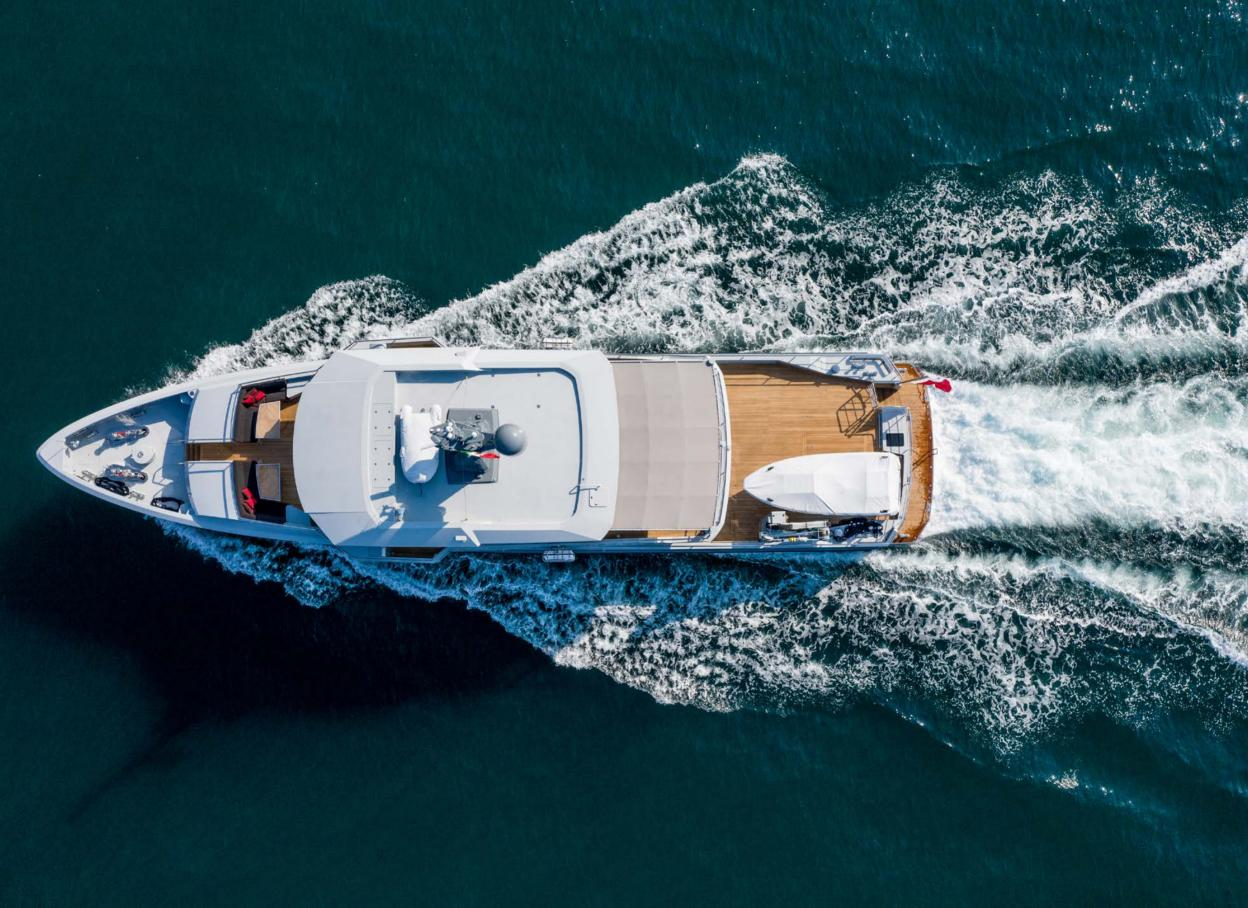
Powered by 2 x MAN D2868 LE 425 engines delivering a top speed of 14.4 knots and a range of 6,000 nautical miles when cruising at 10 knots. Maximum comfort, with noise and vibrations at an incredible low level.
